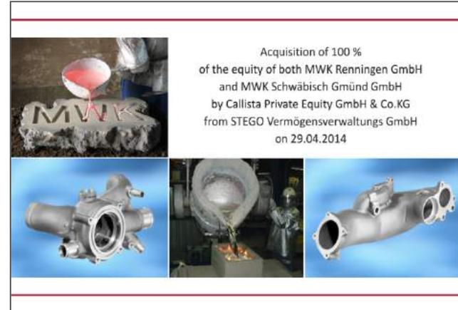
The aluminum foundries – named MWK - are specialized in die casting - LPDC and gravity – as well as sand casting with automated molding lines.
